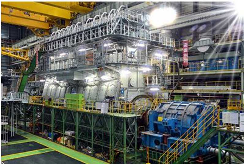
Alternate views of the 11G95ME-C9.5 engine during its shop test in Korea (courtesy Doosan)
