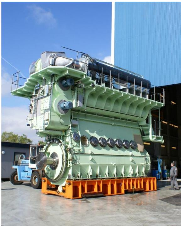
*The world's first, electronically controlled, small-bore, two-stroke engine, a MAN B&W 8S35ME-B, leaving the testbed after successful trials*
