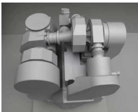
*Model showing the compact architecture of two-stage turbocharging with intermediate cooling*
