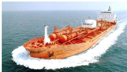
*M/T Bow Firda, delivered in 2003, was the last and most advanced chemical tanker in Odfjell's 37,500 dwt Kværner Class. It is powered by an MAN B&W 7S50ME-C main engine (the world's first) driving a MAN Alpha VBS1560 propeller and shaft alternator*
