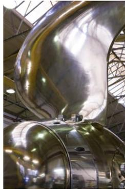
*The optimisation of the VBS Mk 5 includes a new and more streamlined shape of the hub and blade foot integration. The blade foot is completely flush with the hub contour.*
