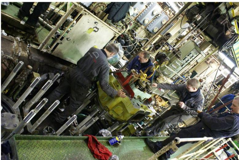
*Cylinder heads are fitted for finishing the engine top section*
