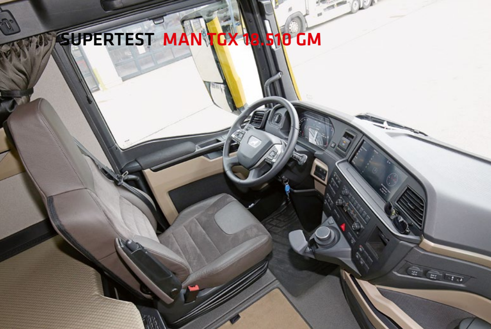
Top steering wheel adjustment; the Smart Select Button is highly user-friendly
